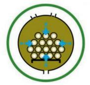
Hydraulic pressure applied, forcing the preservative deep into the structure of the timber.
