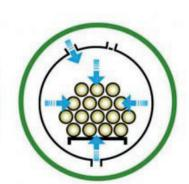
Low pressure inside timber draws in surface solution when vented to atmosphere. Treated timber is left to dry.
